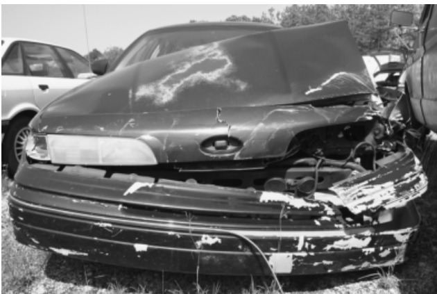
FIG. 2—View of the front part of the 1992 Ford Crown Victoria showing extensive damage to the left headlight and park/turn light assemblies.
