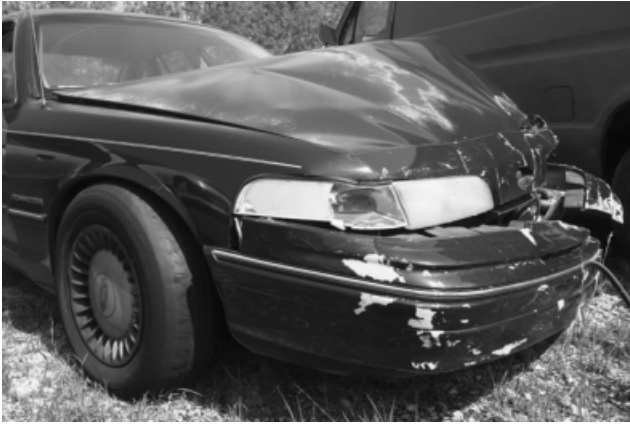
FIG. 1—View of the right front corner of the 1992 Ford Crown Victoria showing damage to the right park/turn light assembly.
