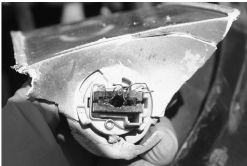
FIG. 4—View of the remnants of the left front park/turn light bulb assembly.
