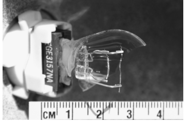
FIG. 3—View of the damaged right front park/turn light bulb.
